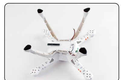
1.9 Congratulations, you have installed the landing gear next let's install the propellers.
