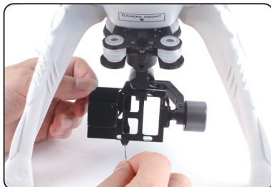
3.5.2 Unscrew 2 M2x4 screw, Loosen the camera fixed frame.
