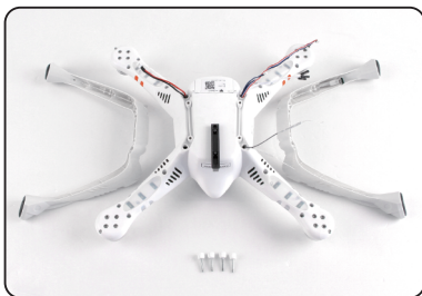
1.1 Prepare quadcopter, landing gear and 4 landing gear fixing screws.
