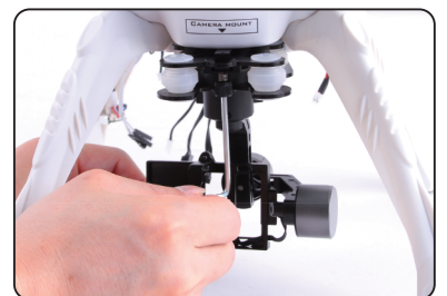
3.3.3 Put the spring into M3x12 screw, aim to the threaded hole, tighten up the screw to Gimbal.
