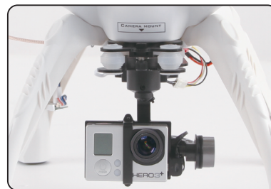
3.5.9 camera and 5.8G emitter installation finished.
