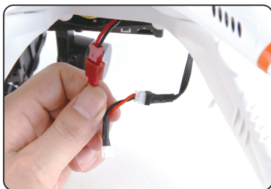
3.5.7 Please connect one mail connector of power conversion line with the gimbal power wire.
