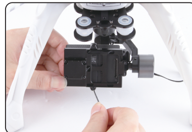
3.5.3 Install the camera into gimbal, Fix it with camera fixed frame (ensure the gap close to the lens), then screw the M2x4 screw to the camera fixed frame again.
