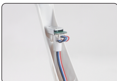
1.7 Secure the cable by pushing it under the "clip" on the compass mounting part.
