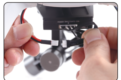
3.3.6 Please connect gimbal power wire with copter power output wire
