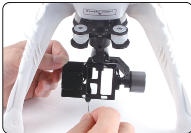
3.4.2 Unscrew 2 M2x4 screw, Loosen the camera fixed frame.
