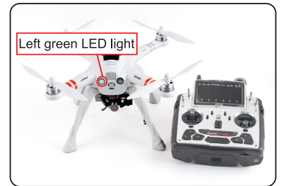
5.6 The left green LED flash quickly till light out which means calibration finished. Please reconnect the aircraft power after calibration.
