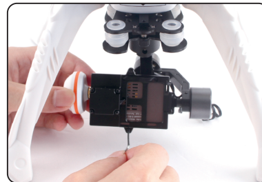
3.4.3 Install the camera into gimbal, Fix it with camera fixed frame (ensure the gap close to the lens), then screw the M2x4 screw to the camera fixed frame again.
