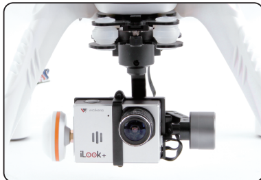
3.4.5 Wiring is done, make sure the camera cable is free so the camera can move freely ,camera installation finished.
