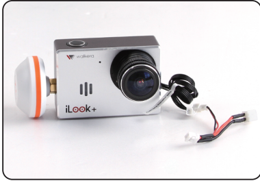
3.2.1 Screw the camera mushroom antenna into Camera.
