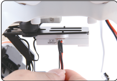
3.2.4 Please insert one mail connector of power conversion line to the power input power of gimbal main control board
