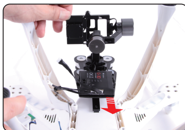
3.3.2 Slide the gimbal onto the mounting track, push on the base until it is all the way back.
