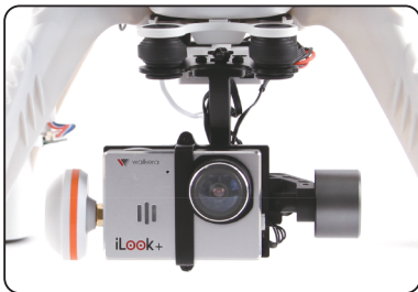
3.2.7 Wiring is done, make sure the camera cable is free so the camera can move freely ,camera installation finished
