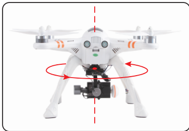
5.4 Horizon level 360° rotation(Rotate the aircraft, from 0° to 90°, 180°, 270°, 360°, all need to pause for 1 second.)
