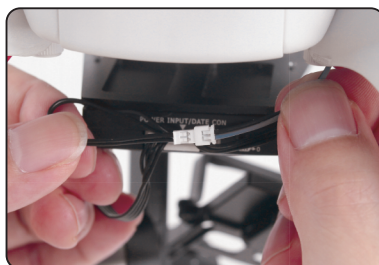
3.3.5 Please connect gimbal video cable with copter video cable
