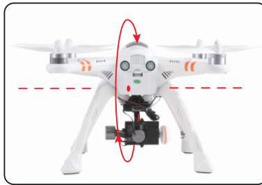
5.2 Forward& backward 360° rotation (Rotate the aircraft, from 0° to 90°, 180°, 270°, 360°, all need to pause for 1 second.)
