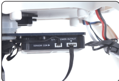
3.4.4 Insert the camera power cable into power output port of G-3D.
