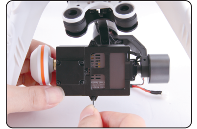
3.2.3 Install the camera into gimbal, Fix it with camera fixed frame (ensure the gap close to the lens), then screw the M2x4 screw to the camera fixed frame again.
