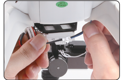
3.2.6 Please connect the camera video cable with copter video signal wire
