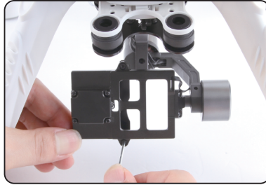
3.2.2 Unscrew 2 M2x4 screw, Loosen the camera fixed frame.
